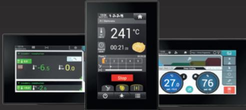
**STM Control Technology** is the STM department that has developed a specific know-how in the **design and production of electronic controllers** for the bakery sector. **Extremely versatile and fully customizable** control systems, which allow full machine supervision, parameter optimization and complete control even remotely thanks to the **STM-Cloud System**.
